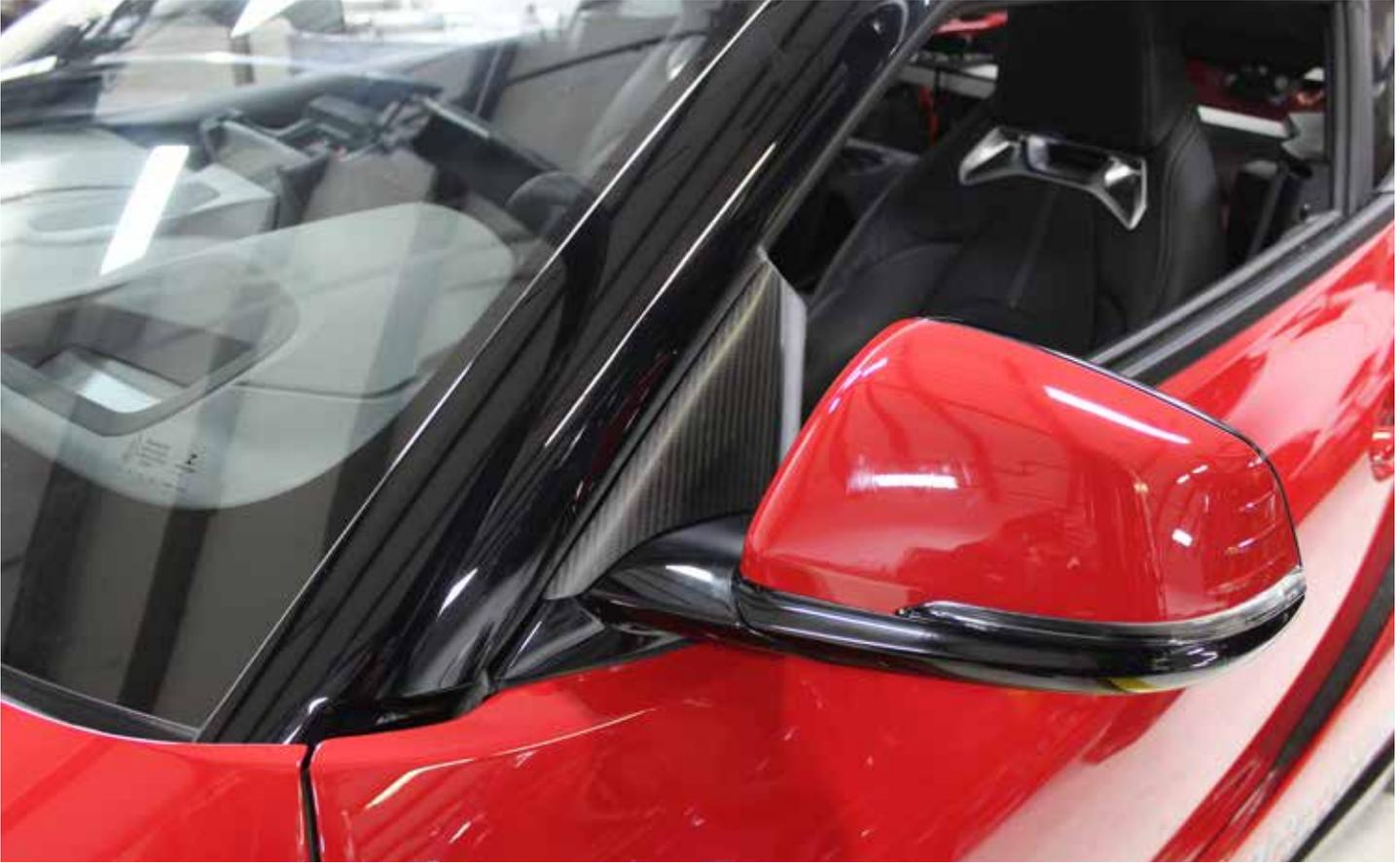
**3)** Clean off the mirror base with isopropyl alcohol and let dry. It is very important that the surface of the mirror is clean before installing the plates.
