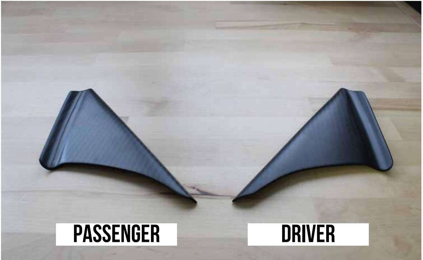
**2)** Test fit the drivers wind deflector on the mirror base to get an idea where it will sit.
