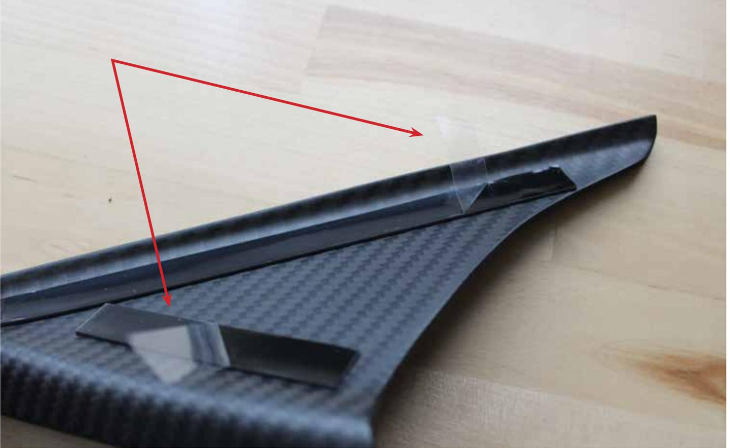
**5)** Lightly position the wind deflector on the mirror base keeping the adhesive backing accessible to grab from the edges.
