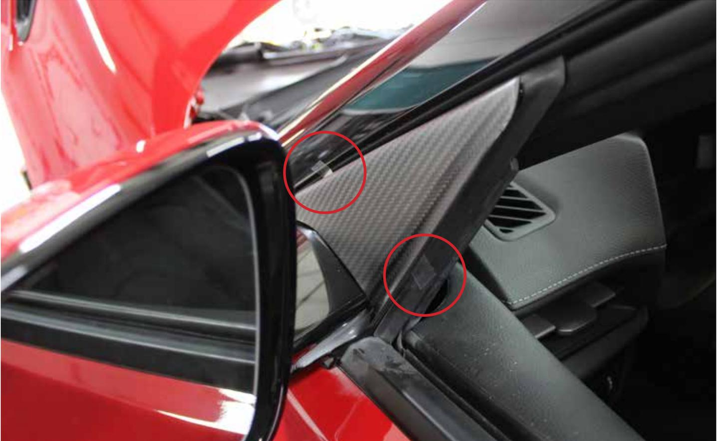
**6)** Once in position, lightly hold the mirror plate with one hand and pull the rest of the backing off with the other. Apply a reasonable amount of pressure to permanently adhere the wind deflector to the mirror base.
